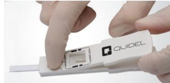
Snap the sample collector into the Test Cassette.
