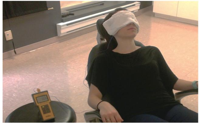
**Fig. 1.** Experimental set-up. The thermometer probe was secured to the lid with surgical tape such that the end of the probe was directly under the mask/cloth. The temperature could be read from an external digital reader.
